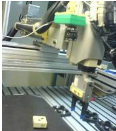
Figure 2: Position of the camera mounted on the vertical axis of the robot
