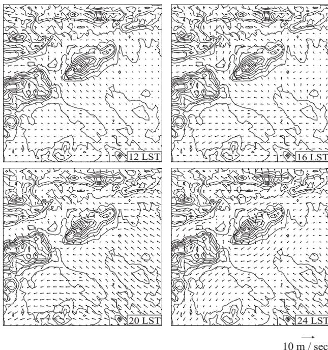
Fig. 2; Simulated surface wind fields (10 m AGL) for the fine domain at 12, 16, 20 and 24 LST for the 20<sup>th</sup> of July 2004.
