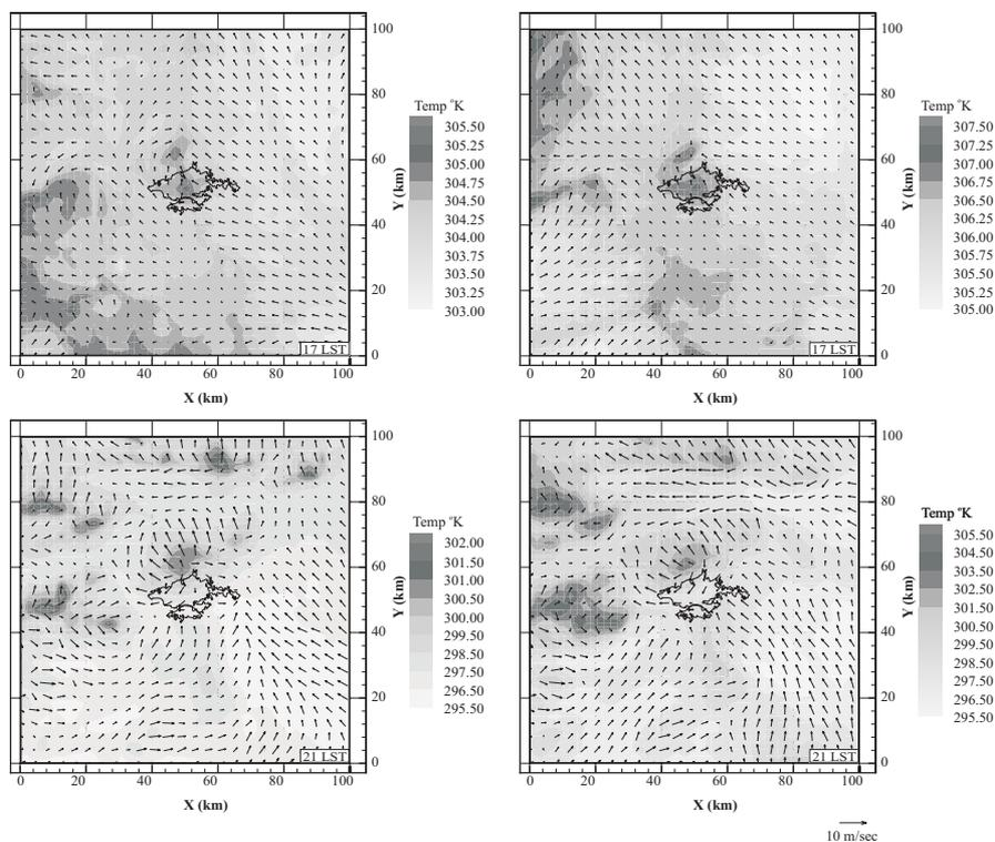
*Fig. 3; Simulated surface wind fields (10 m AGL) and temperature isopleths ( $^{\circ}$ K) at 150 m ASL, for the fine domain at 17 and 21 LST for the 10<sup>th</sup> of June (left) and the 21<sup>th</sup> of July (right) 2004. The city of Zagreb is outlined.*
