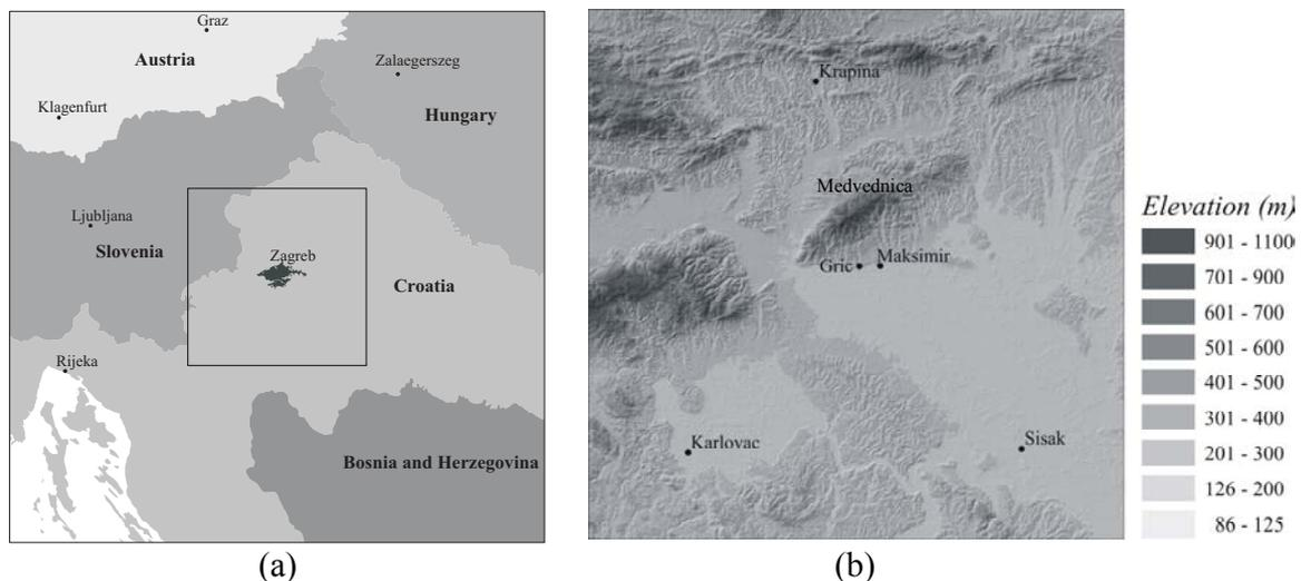
Fig. 1; (a) Configuration of nested grids. The outer frame indicates the coarse grid and the inner one the fine domain. (b) Anaglyph for the fine grid. The bullets indicate the positions of the routine measuring sites. The domain centre is in Zagreb (Latitude  $45^{\circ} 48' 15''$  N, longitude  $15^{\circ} 58' 29''$  E), 150 m above sea level, located in the foothill of mountain Medvednica.
