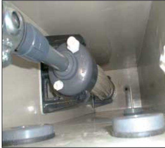
Fig.1. Top view of Zenon (ZW 10) hollow-fiber microfiltration membrane bioreactor.
