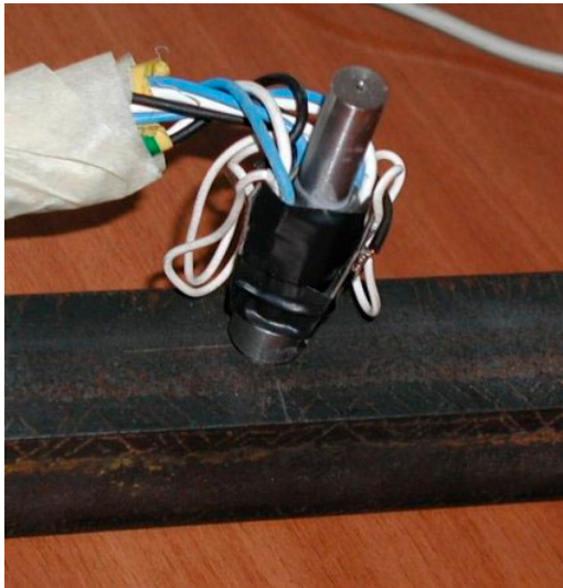
Figure 2. Force-measuring device (indenter)
