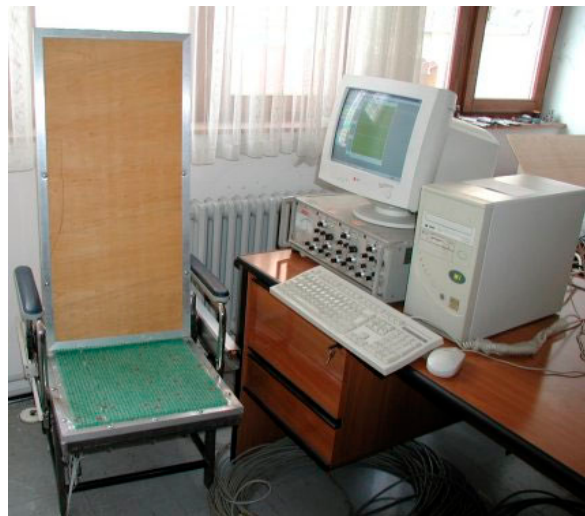
Figure 3. The equipment used to measure sitting pressure
