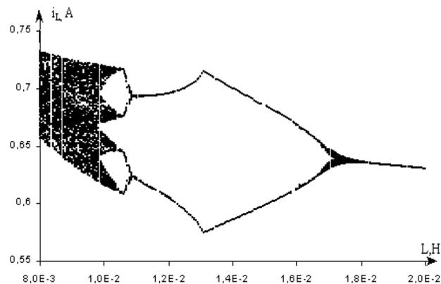
Fig.3. Bifurcation diagram with the load inductance as the bifurcation parameter ( $E=22\text{V}$ ,  $T=330\mu\text{s}$ ,  $\Delta L=50\mu\text{H}$ )
