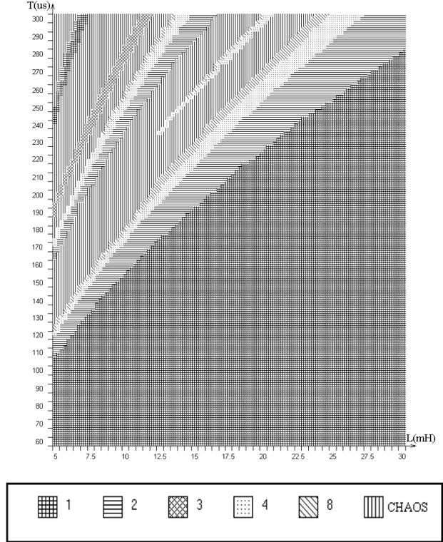
Fig.7. Load inductance vs. period of the external sawtooth ramp voltage ( $LT$ ) bifurcation diagram ( $E=22V$ ) representing zones of period- $N$  operation and chaos ( $N=1,2,3,4,8$ )
