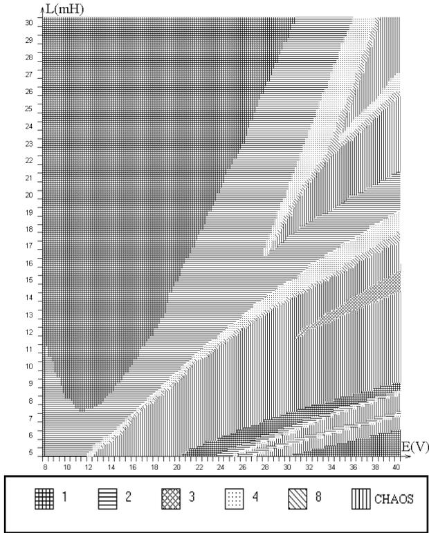
Fig.5. Input voltage vs. load inductance ( $EL$ ) bifurcation diagram ( $T=330\mu s$ ) representing zones of period- $N$  operation and chaos ( $N=1,2,3,4,8$ )
