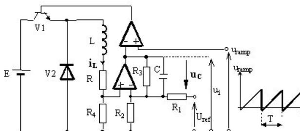
Fig.1. Functional diagram of the buck converter
