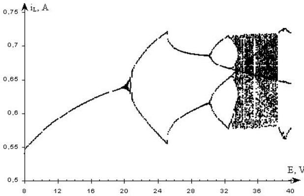
Fig.2. Bifurcation diagram with the input voltage as the bifurcation parameter ( $L=15\text{ mH}$ ,  $T=330\mu\text{s}$ ,  $\Delta E=0.1\text{V}$ )
