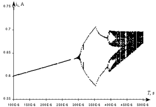
Fig.4. Bifurcation diagram with the period of external sawtooth ramp voltage as the bifurcation parameter ( $E=22\text{V}$ ,  $L=15\text{mH}$ ,  $\Delta T=1\mu\text{s}$ )
