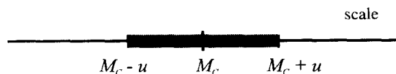
Fig. 1. The result of measurement of quantity M is a range of values expressed by the best estimate of the quantity ( M_c ) and the uncertainty ( u ).
