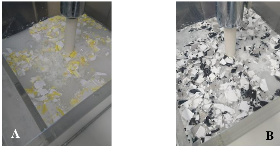
Fig. 4: Flotation process of paper with a) yellow and b) black labels
