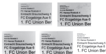
Fig 6. Enlarged images of positive text: a) HP Indigo to Thermoeco substrate; b) Durst to Thermoeco substrate; c) HP Indigo to PP substrate; d) Durst to PP substrate; e) the original display screen (monitor).
