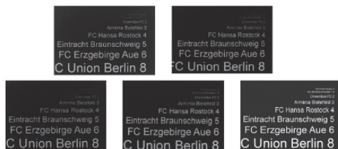
Fig 7. Enlarged images of negative text: a) HP Indigo to Thermoeco substrate; b) Durst to Thermoeco substrate; c) HP Indigo to PP substrate; d) Durst to PP substrate; e) the original display screen (monitor).
