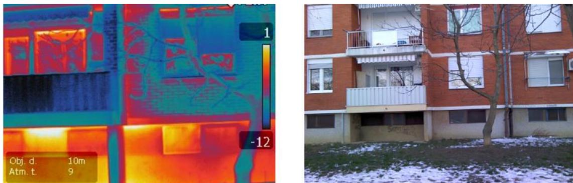
Figure 6. Building envelope thermal image of Building C
