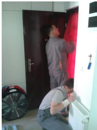
Figure 1. Airtightness measurements by using a Minneapolis Blower Door equipment
