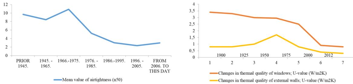
Figure 2. Mean value of airtightness ( $n_{50}$ ) according to periods of construction and changes in thermal quality of windows and external walls
